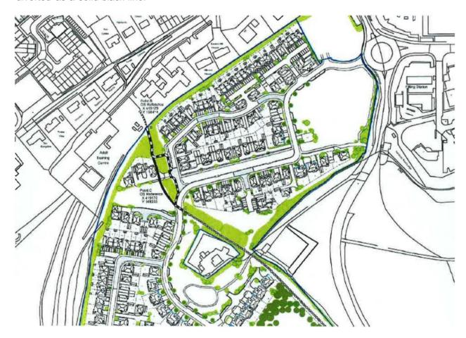
3.4 The proposed diversion will divert a 65 metre section of path and create 75 metres of path. The new route will be laid to tarmac and hoggin (a compactable groundcover that is composed of a mixture of clay, gravel, and sand or granite dust that produces a buff-coloured bound surface). The sections of footpath MARL30 that are within the development site, but do not need to be diverted, will also be improved with a surface of hoggin and a width of 2 metres will be provided.
